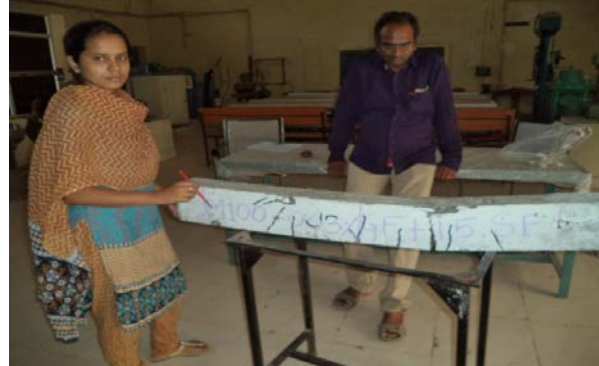
Plate No 1 : Failure modes of Hybrid fibre High Strength Reinforced Concrete Self Compacted Beams
